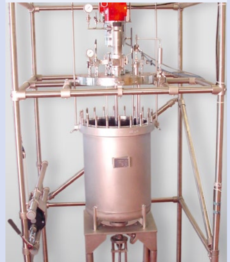
100 liter 50 bar hydrogenation reactor 100 Liter 50 bar Hydrier Reaktor
