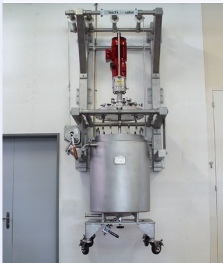
100 liter, 60 bar hydrogenation reactor, Hastelloy, cGMP, wall mounted 100 Liter 60 bar Hydrierreaktor, Hastelloy, cGMP, Wandmontage
